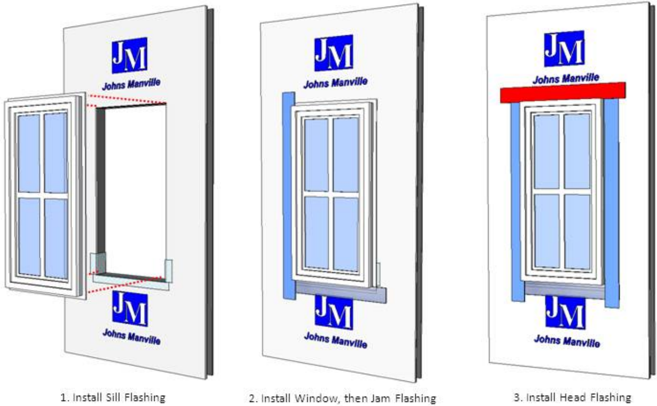
FIGURE 4. TYPICAL PENETRATION FLASHING DETAIL - FLANGED
